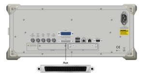
Figure 2.6.4-1 Output connector location
